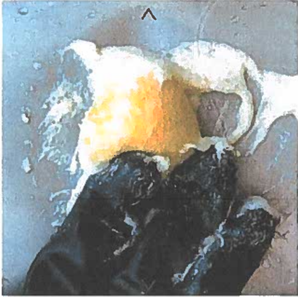
drum leak golf ball plug
