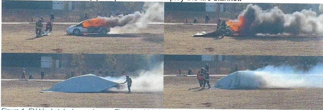
Figure 1. EV blanket deployment on an Electric vehicle in thermal runaway. Courtesy Stephens Truck Center
