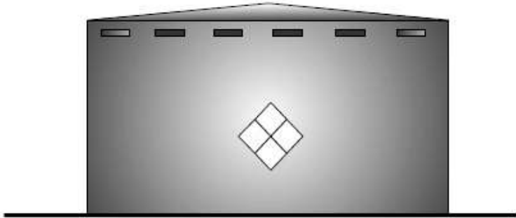
Covered Top Floating Roof Tank Flammable and Combustible Storage
